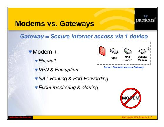
As we mentioned in the beginning of this presentation, a Gateway typically consists of a modem <u>plus</u> a firewall, VPN, NAT Router and management functionality.
