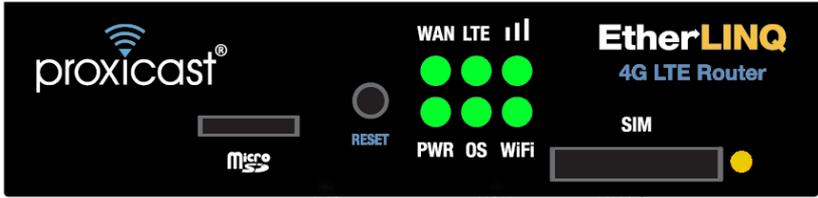
Figure 2: EtherLINQ Front Panel
