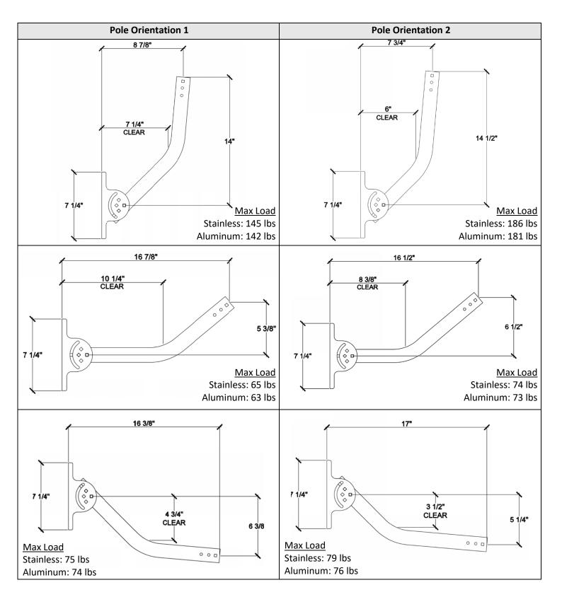
© Copyright, Proxicast LLC. All rights reserved. Max loads calculated with Locking Bolt installed Rev 20230418
