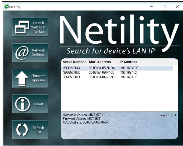
The **Network Settings** button allows you to configure the IP address and related network parameters of the MSNSwitch as well as set the password. The **Launch Web User Interface** button will open the MSNSwitch's internal web server in your default browser.
