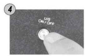
Step 4: Press and hold UIS ON / OFF button (2 seconds) to enable Auto Reset function.
