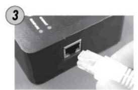
Step 3: Connect LAN cable from Router. The Internet LED will turn ON to indicate online.
