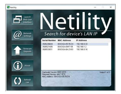
The **Network Settings** button allows you to configure the IP address and related network parameters of the MSNSwitch as well as set the password. The **Launch Web User** Interface will open the MSNSwitch's internal web server in your default browser.
