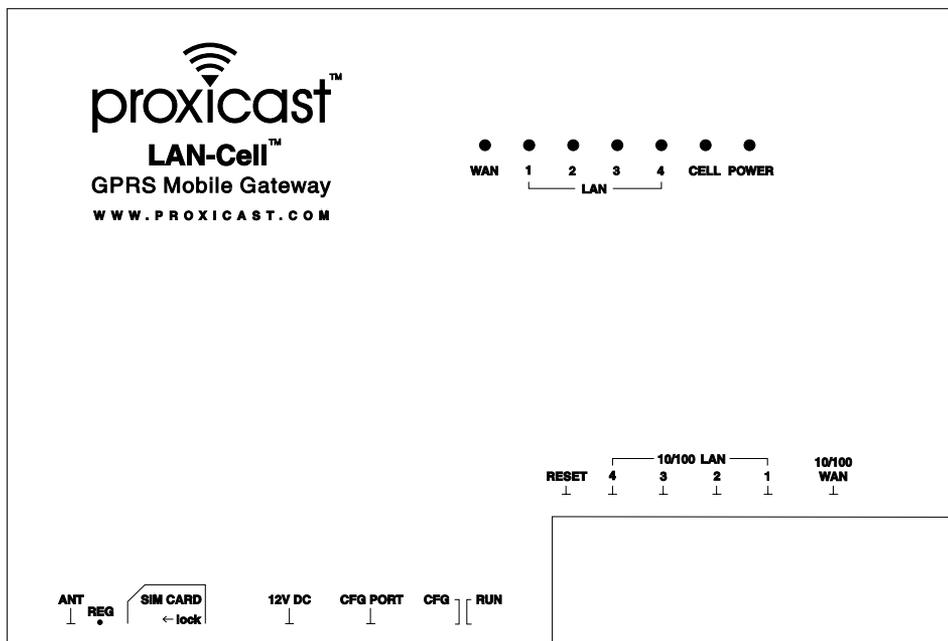
Figure 1: LAN-Cell GPRS Mobile Gateway (Model GPRS-401)
